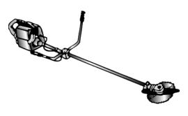
*Safety tip:* The open blade is on the end of a wand, and can snag and swing violently to the side, making it more prone to injure other workers rather than the operator. Other workers should stay clear.
